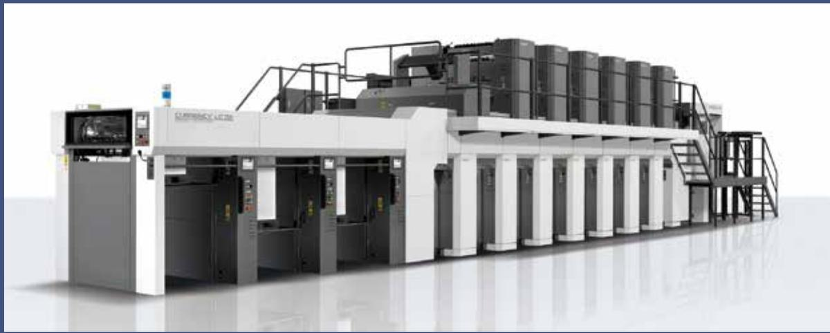
The Currency IC532/// is a five-color indirect intaglio sheetfed press equipped with a nonstop feeder and two delivery piles along with one delivery sampling pile for continuous production at the maximum printing speed of 10,000 sheets per hour.
