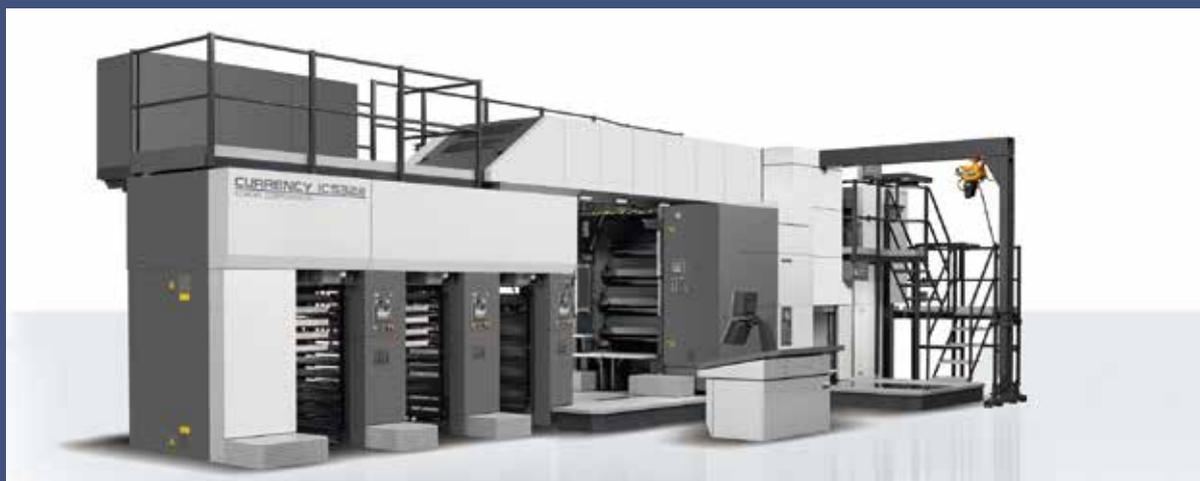
Komori's numbering press, the Currency RN332///, is a three-color machine featuring a double-size common impression cylinder, a photopolymer plate cylinder, and an inspection cylinder that works together with a high precision inspection camera.
