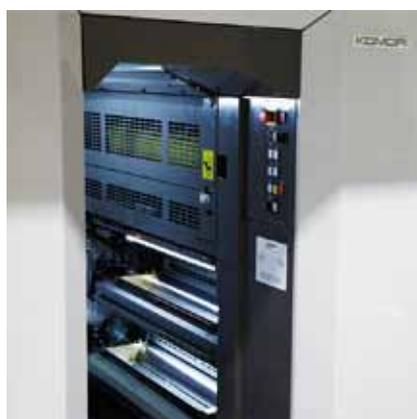
Lower deck printing unit of the LC-1232 double-deck multicolor offset press showing how accessible the lower units are. Inking ducts can be seen at the lower end of the unit.
